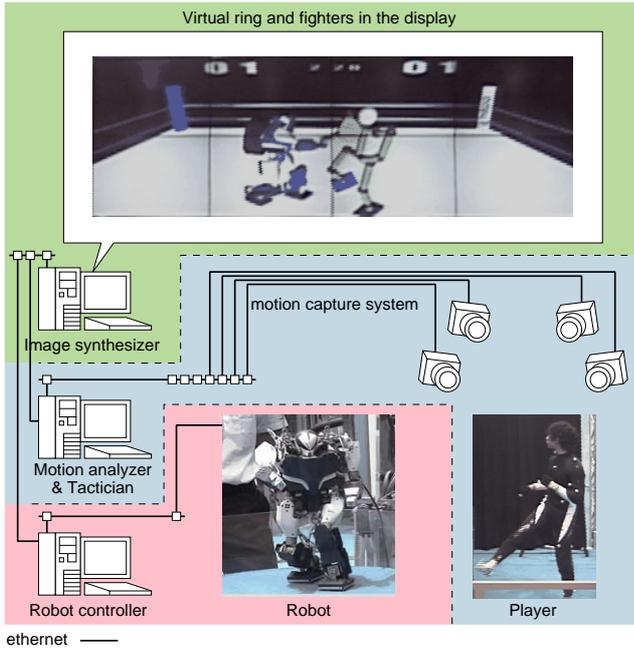
Fig.7 Diagram of virtual fighting system
