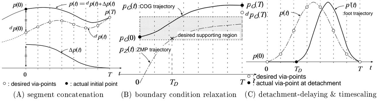
Fig.11 Interpolation toolbox for physically consistent motion trajectory
