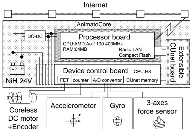
Fig.5 Electronics system of UT- $\mu$ 2
