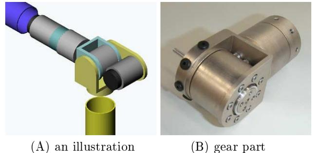
Fig.3 Ortho-axis-coupled joint unit
