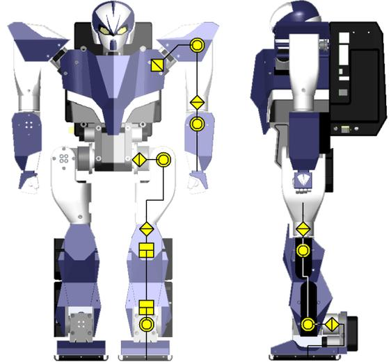
Fig.2 Joint assignment of UT- $\mu$ 2
