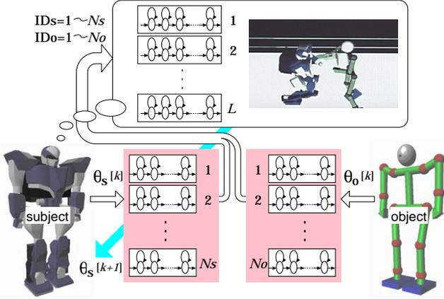
Fig.9 Mimetic communication with hierarchical HMM
