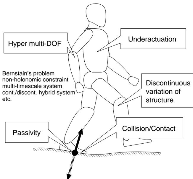
Fig. 1. Dynamical properties of humanoid systems
