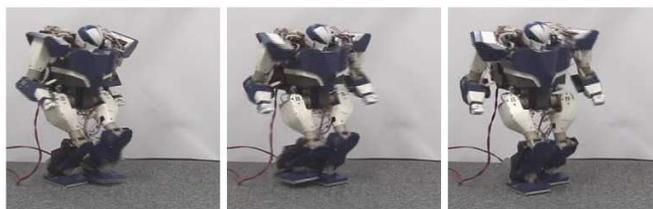
Fig. 3. Walking (0.3[s/step]) by UT- $\mu$ 2
