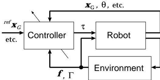
**Figure 3:** Humanoid control system connected with environment
