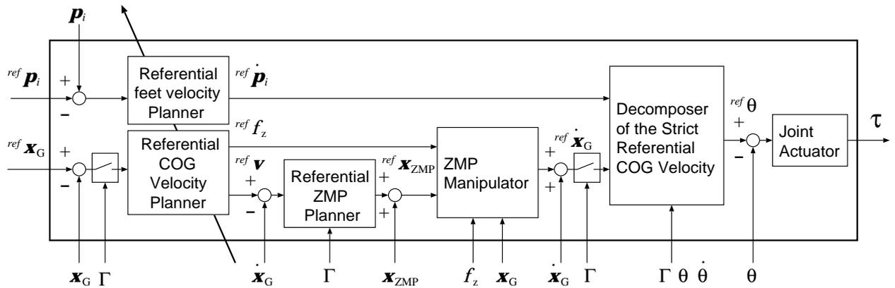
Figure 4: Block diagram of a humanoid controller
