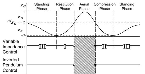
**Figure 2:** Contact phase, impedance and inverted pendulum control
