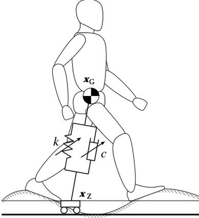
**Figure 1:** Legged system and variable impedant inverted pendulum
