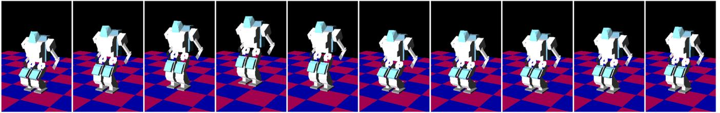
Figure 6: Snapshot of a jump motion simulation
