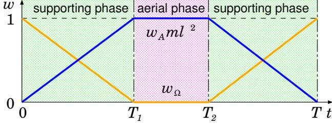
Fig. 3. Variable weight in accordance with contact phase
