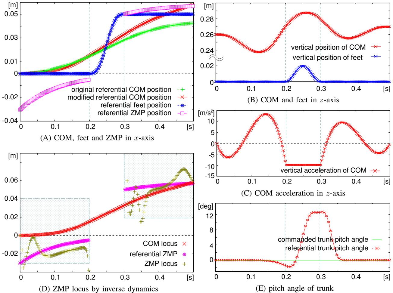
Fig. 6. Planned trajectory of COM, foot and ZMP
