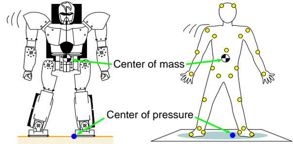
Fig. 1: COM-ZMP model highlights common principle in dynamics of human-formed mechanical systems
