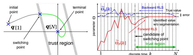
Fig. 4: Identification of trust region and parameters utilizing RLS
