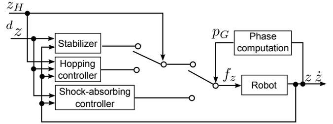
Fig. 9. A block diagram of the controller enabling transition of standing, hopping and shock-absorbing
