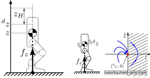
Fig. 1. Mass-concentrated model of a biped robot
