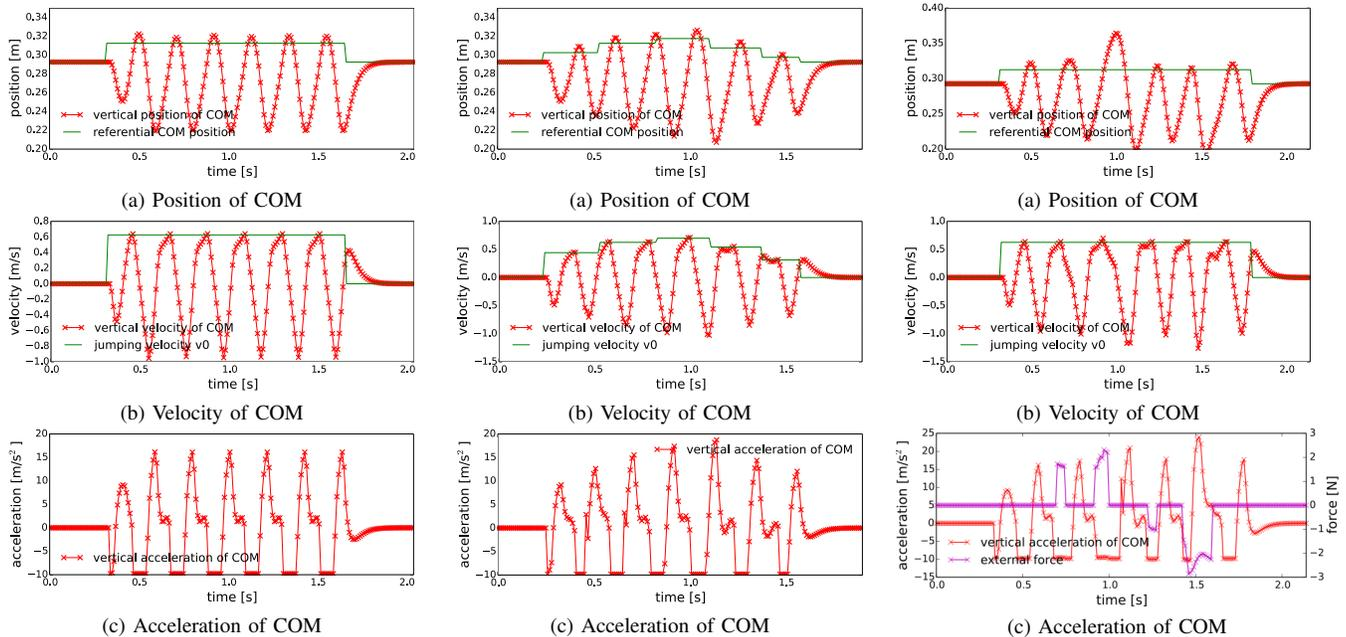
Fig. 11. Results of the simulation. The desired hopping height was set to  $z_H = 0.02$ [m].
