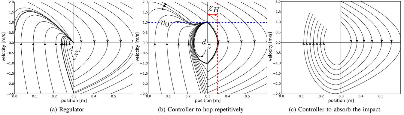
Fig. 5. Phase portraits of the system in the case of using each controllers. (a): The regulator defined by Eq. (4) is applied. The point  $(^dz, 0)$  on the phase plane should be stable equilibrium. (b): The controller defined by Eq. (7) is applied. The state on the phase plane should converge to  $(^dz, v_0)$  for stable hopping. (c): The controller defined by Eq. (15) is applied. The state on the phase plane should traverse smoothly.
