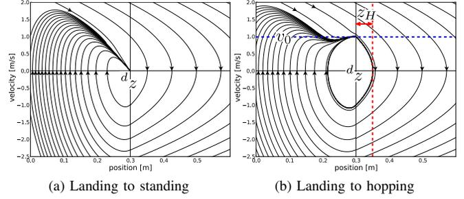
Fig. 8. Phase portraits of the system. (a): Solid line represents the direction of the eigenvector of the regulator. (b): Horizontal dashed line represents  $v_0$ . Vertical dashed line represent the desired hopping height  $z_H$ .
