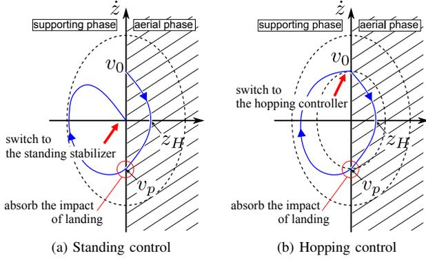
Fig. 6. Trajectories of COM in the phase space. In the standing control as well as the hopping control, the controllers need to be designed to absorb the impact of landing.
