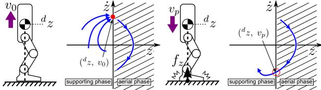
Fig. 2. A moment that the robot lifts off at  $\dot{z} = v_0 = \sqrt{2gz_H}$
