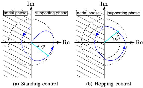
Fig. 7. Trajectories of the complex number  $p_G$  on the complex plane.  $\phi$  is the argument of  $p_G$ .  $\alpha$  is the angle between the real axis and the direction of the eigenvector.
