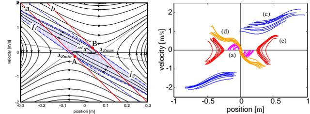
Fig. 1. Phase portrait of COM-COP regulator and measured loci
