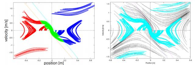
Fig. 2 Identified segments of the piecewise-affine system
